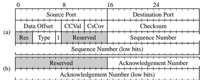
**Figure 2:** DCCP packet header. The generic header (a) begins every DCCP datagram. Individual packet types may add additional information, such as (b) an acknowledgement number. The packet header is followed by DCCP options, then payload; payload starts Data Offset words into the datagram.
