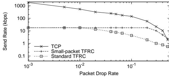
**Figure 7:** Send rate for given packet drop rates using TCP, standard TFRC, and small-packet TFRC. TCP uses bulk transfer and 1460-byte segments; TFRC uses 14-byte segments and has an application-limited maximum send rate of 12 kbps including headers.
