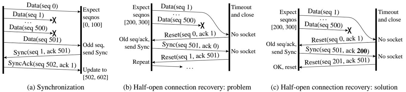
Figure 3: Recovering synchronization after bursts of loss.
