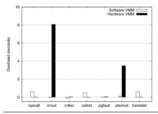
Figure 5. Sources of virtualization overhead in an XP boot/halt.
