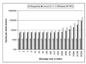
Figure 5: Send-receive cost vs. buffer size
