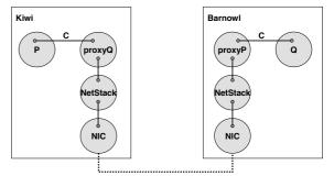
Figure 4: Cross machine channel via TCP proxy
